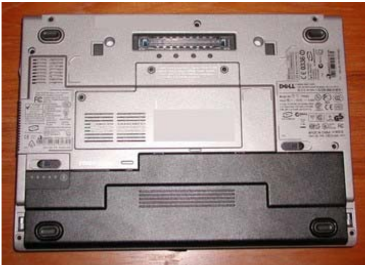
Underside view of the D420: Expansion Slot, Battery (hard drive accessible underneath), Memory Upgrade Slot (under panel) ( view large image )
