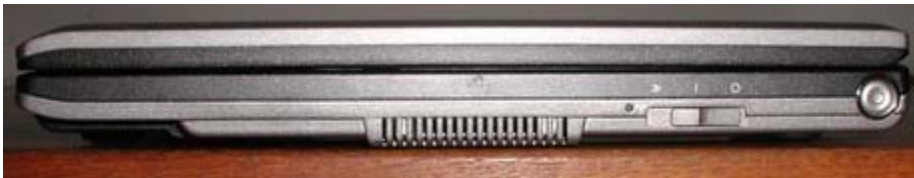
Right side view of ports on the D420: Wi-Fi Catcher, Fan Vent (view large image) ( view large image )
