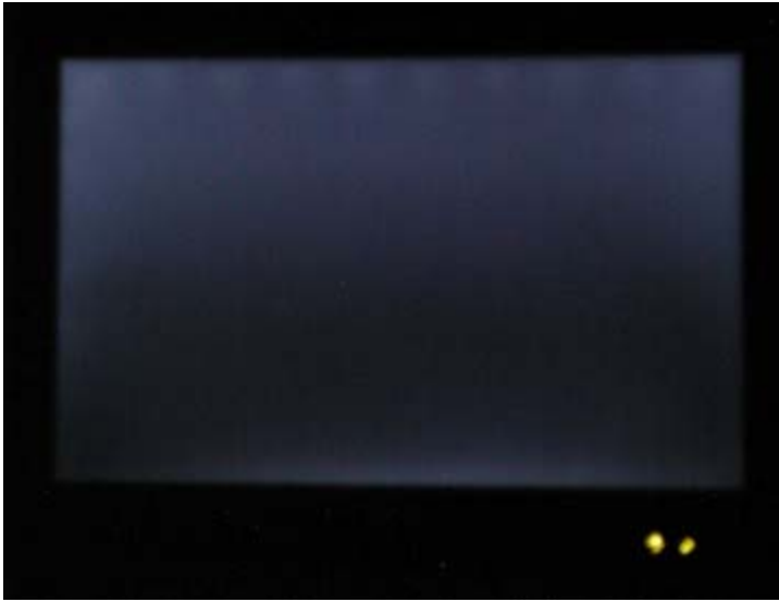
Minimal light leakage found on the D420 AU Optronics screen ( view large image )
