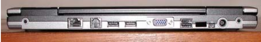
Back side view of ports on the D420: Ethernet LAN RJ-45, Modem RJ-11, 2 USB 2.0 Ports, VGA Out, D-Bay USB Port, IEEE1394 Port, Power Port (view large image) ( view large image )
