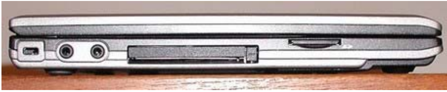
Left side view of ports on the D420: Kensington Lock, Microphone Out, Headphone Out, PCMCIA Slot, SD Card Slot (view large image) ( view large image )
