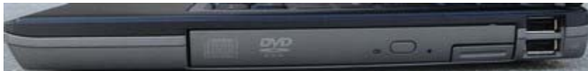
Right side view of ports on the D620: Optical drive media bay (removable and swappable), 2 USB 2.0 ports ( view large image )
