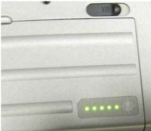
The battery has a built-in charge indicator on the D620 ( view large image )
