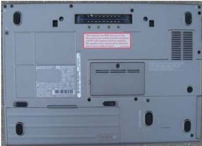
Underside view of the D620: Expansion slot (at the back), battery (at the front), memory slot in the middle ( view large image )
