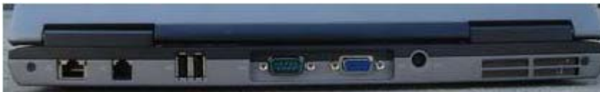
Back side view of ports on the D620: Ethernet LAN and Modem, 2 USB 2.0 ports, Serial port, VGA out port, Power port, Fan and Vents ( view large image )
