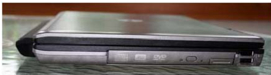
The right side. Only a DVD Burner and two USB slots ( view large image )
