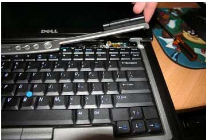
Removing the hinge to get to RAM slot ( view large image )
