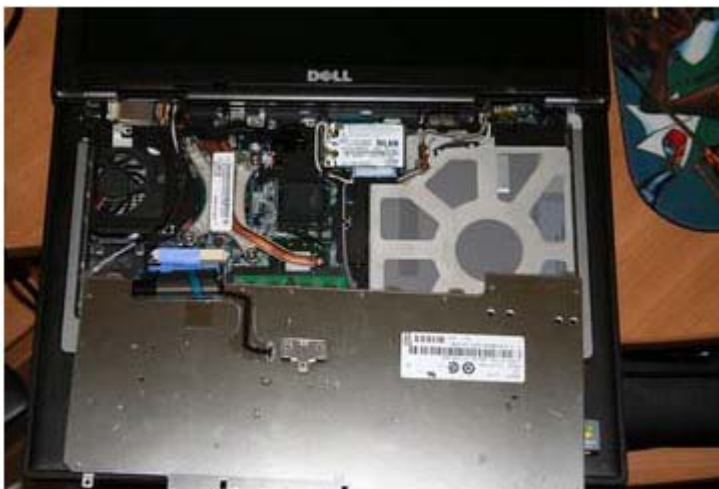
Access to memory slot ( view large image )
