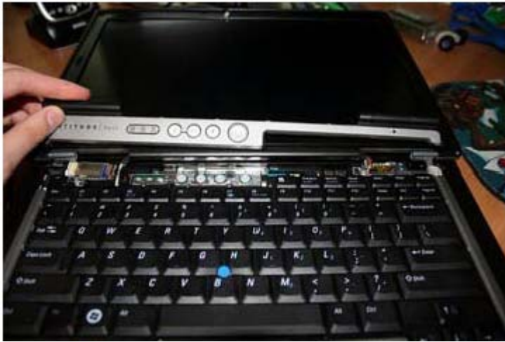
Hinge removed ( view large image )
