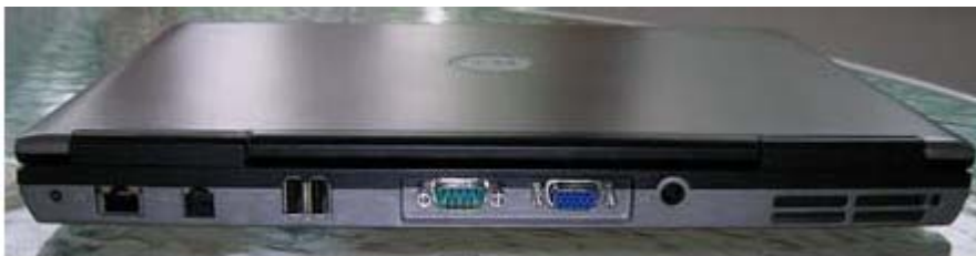
The back of the machine including a serial port for old devices. ( view large image )
