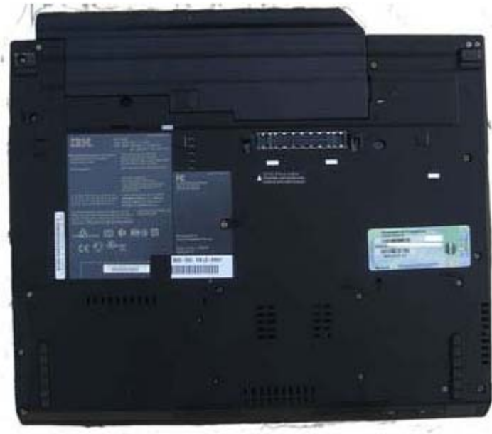
T60 underside view: Port replicator connector, access to memory, battery release latch and lock ( view larger image )
