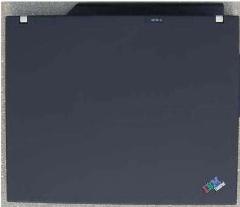
Above view -- the same ThinkPad look as ever except that hump on the right which contains the WWAN antenna on this specific model (if you order a T60 without WWAN connectivity you will not have this)
